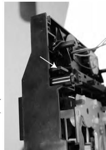
When a disc is loaded, unlock the tray by pushing the slide inwards with a screwdriver and pull tray outwards.
